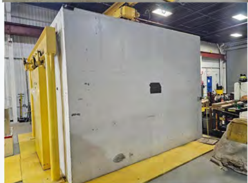
Alaron's shielded hot cell with telemanipulator arms.
