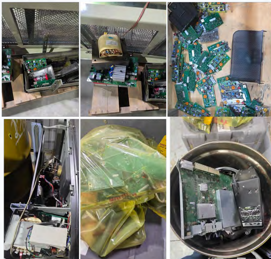
Recovered circuit boards staged for survey and free release at the WCS Alaron Facility.
