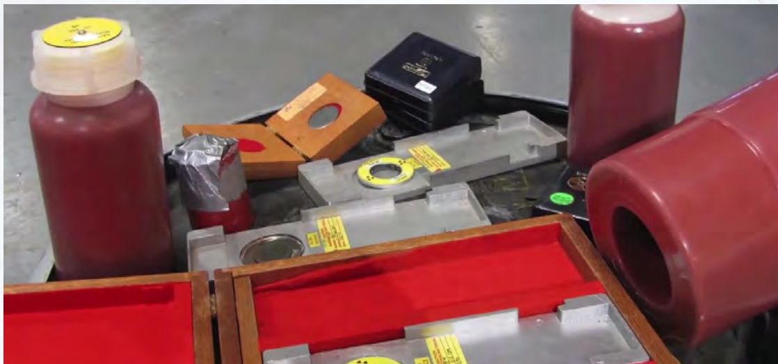
Sealed source containers staged for processing at the WCS Alaron Facility.
