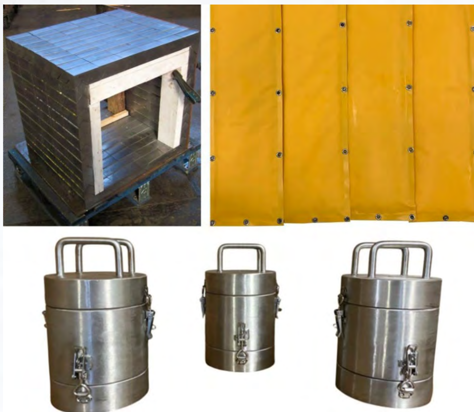
Lead bricks, blankets, "pigs" and debris staged for recovery and recycling.
